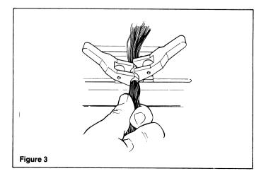
**NOTE:** When using bundles of individual discrete wires, be sure that the portion being grasped by the clamps is taped to protect the insulation and aid in retaining the wires. (Figure 4)
